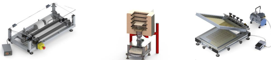
Fig. 2. Ball-mill (left), TGA (middle) and screen printer (right) developed by Fiaxell
